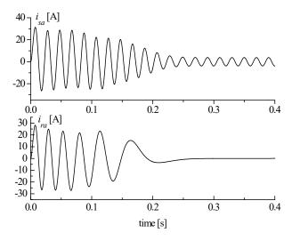
Fig.4. Stator and rotor current during free acceleration
