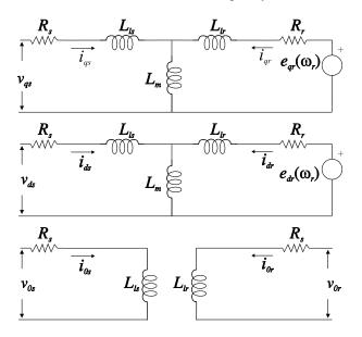
Fig.1. Induction motor equivalent circuit
