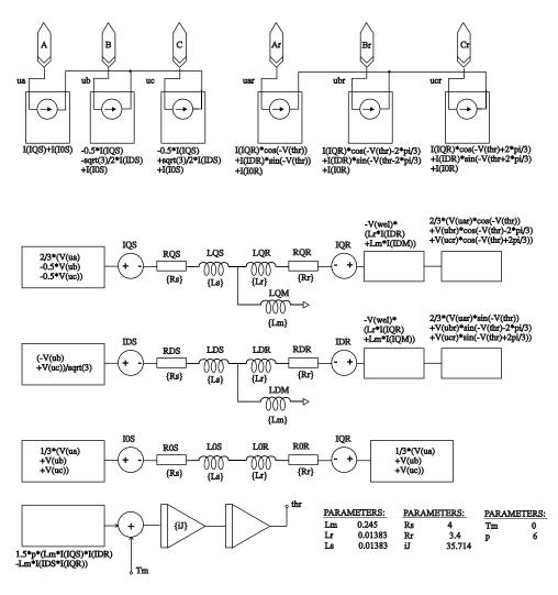
Fig.2 Induction motor model for PSPICE
